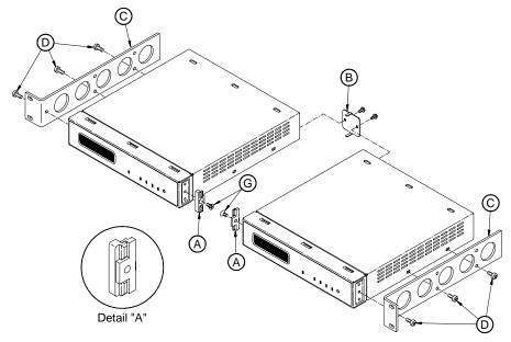
Using Pozidriv screwdriver, attach Rack Ear-Full Rack (C) to each E5810 with six M4x10 Panhead Screws (D).
