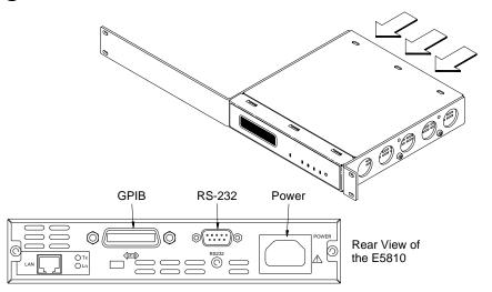
Using Phillips screwdriver, attach Rack Ears to rack with four Machine Screws (D) and four Machine Nuts (E).
